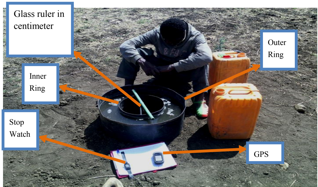
Figure 3.12: Field measurement of infiltration capacity using double-ring infiltrometer
