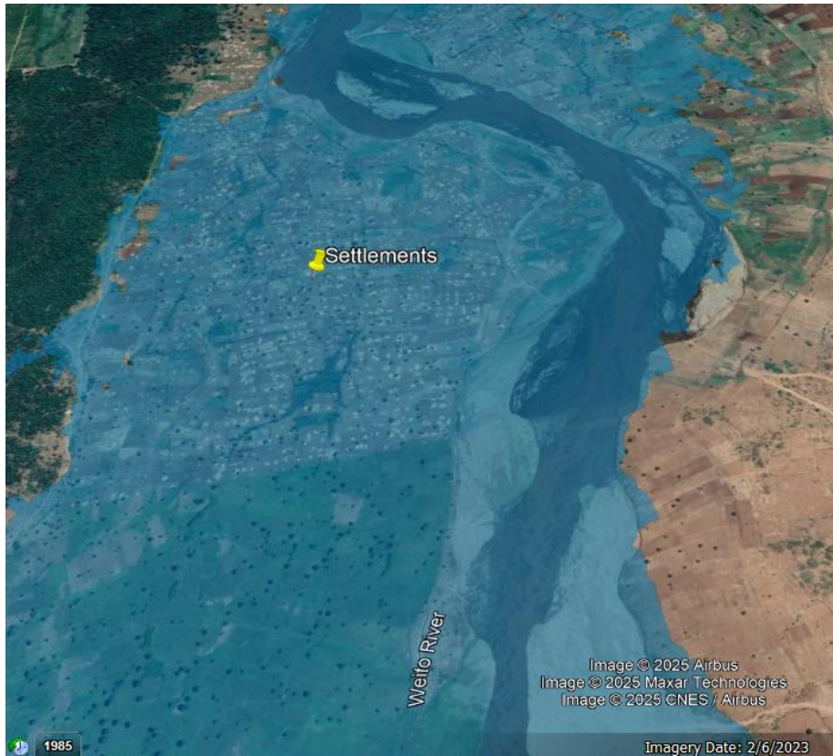
Figure 4.10: Rural settlements under 100 years flood
