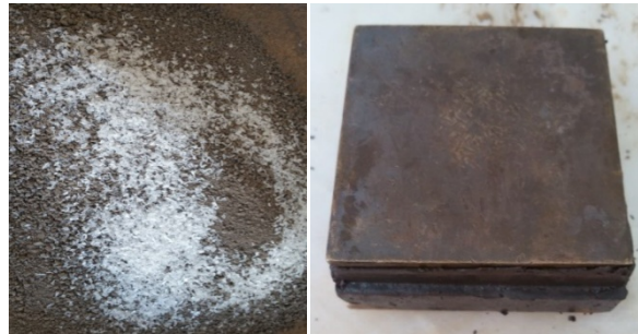
Figure4. 11 The mixture of soil sample with flexi and the shear failure point
