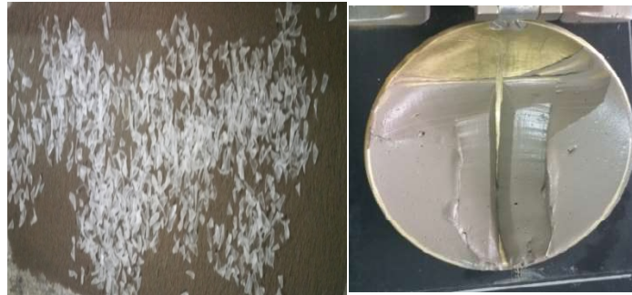
Figure3. 4 Random mix of black cotton soil with flexi and the jointed sample at the cup
