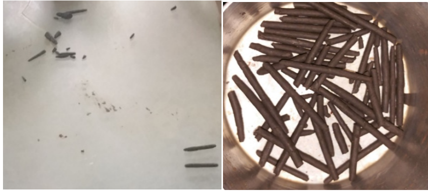
Figure4. 4 plastic limit of flexi stabilized soil
