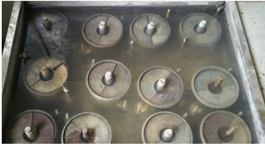
Figure4. 10 Modified CBR soil sample for all stabilizer content during soaked period
