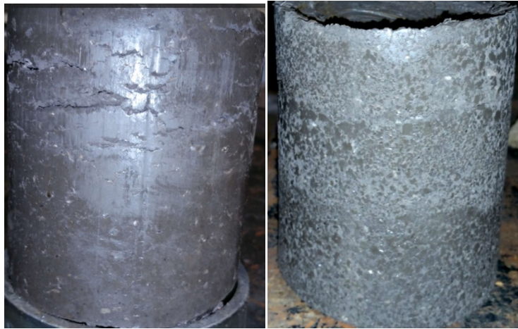
Figure4. 8 Optimum flexi stabilized soil sample of standard and modified compaction
