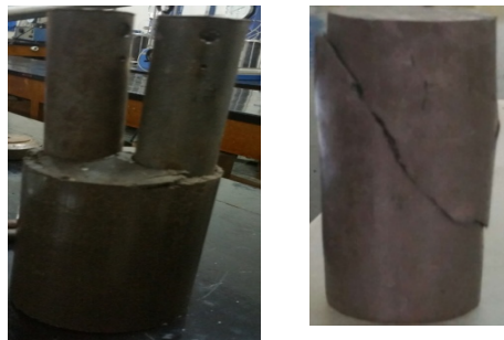
Figure4. 15 UCS remolded sample and failure of 2% flexi stabilized black cotton soil
