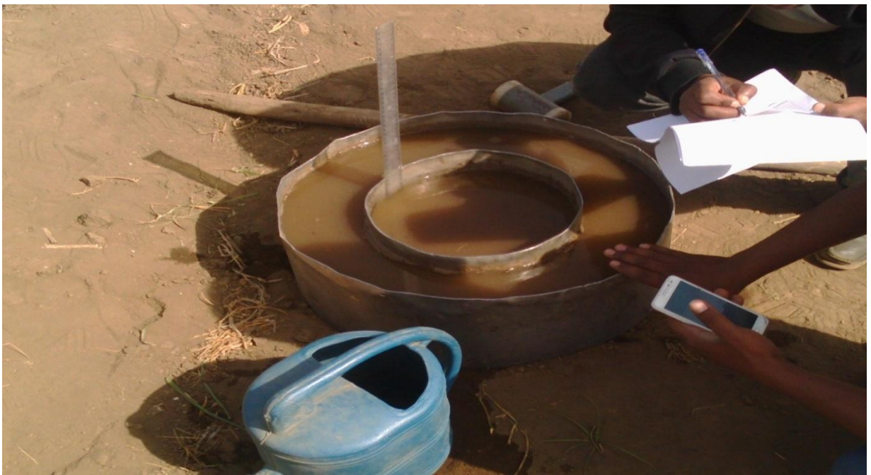
Appendix figure 2. Recording of infiltration depth to determine basic infiltration rate
