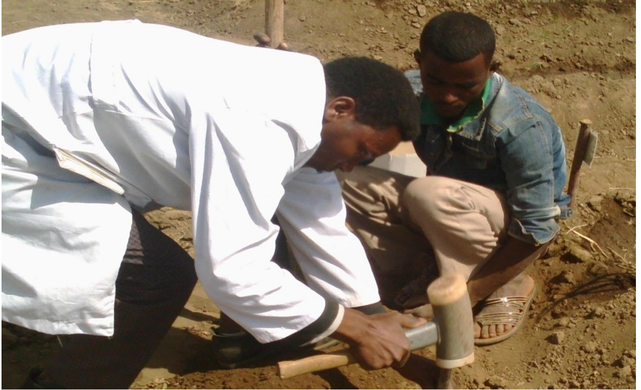
Appendix figure 1. Taking soil sample to determine bulk density and other parameter
