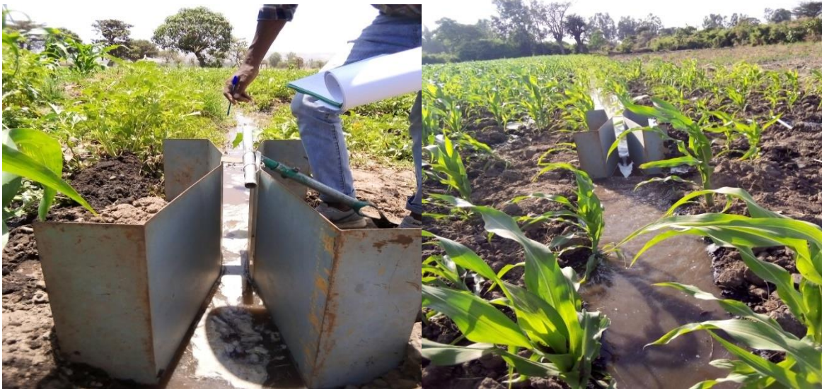
Figure 3.11: Measurement of Field Applied Irrigation Water using Parshall Flume
