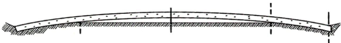
Figure 2. 3 Outdoor slabs exposed to the sun, curl downward (Ytterberg, 1992).
