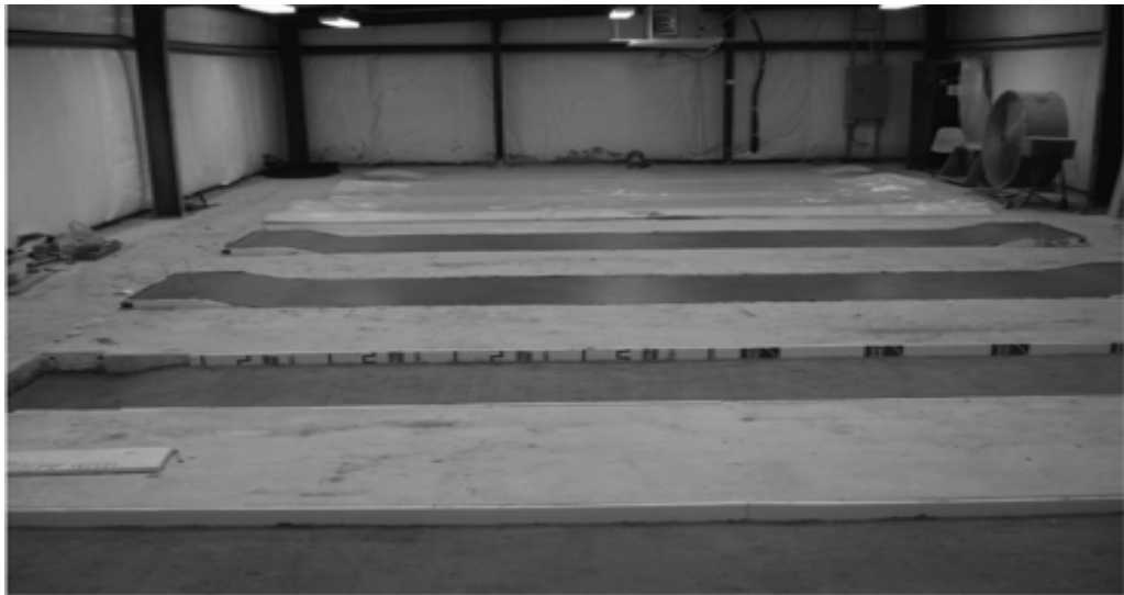
Figure 3. 6 Slab-on-ground test set-up for shrinkage validation ( Shadravan et al., 2015 ).
