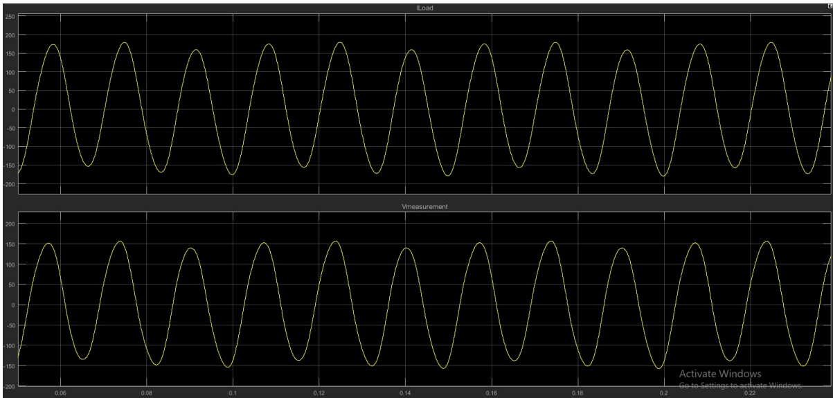
Figure. 5.38. Output of voltage and current inverter with filter
