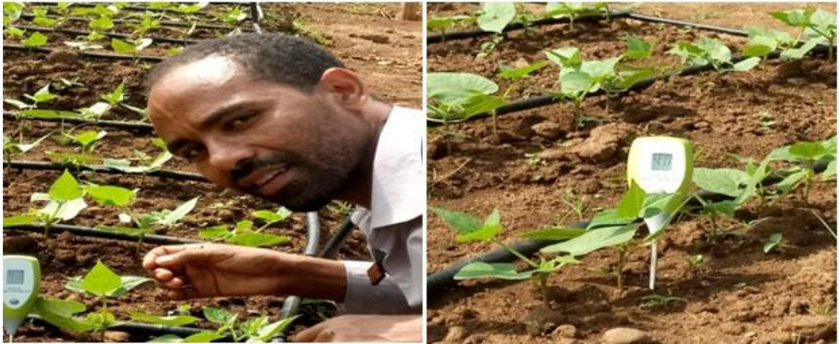
Figure 7: Soil moisture measurement using Digital Moisture Meter
