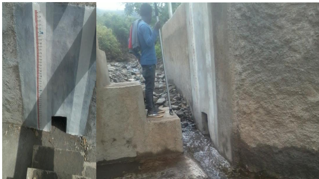
Appendix Figure 3: Flow depth and velocity measurement at hydrological weir using stage reading and current meter
