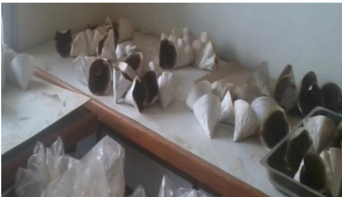
Appendix Figure 4: Filtering and drying sediment sample in the laboratory
