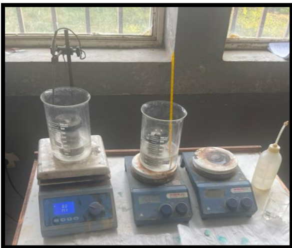
Figure 3. 2: Colorless chemical bath solution before 10 minutes and chemical composition
