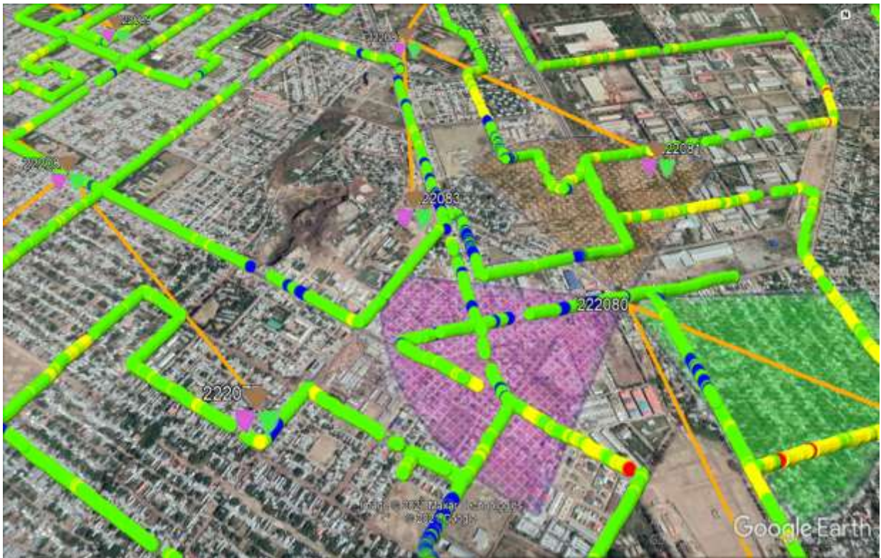
Figure 4.4 Sample drive test of 1800 MHz displayed on google earth
