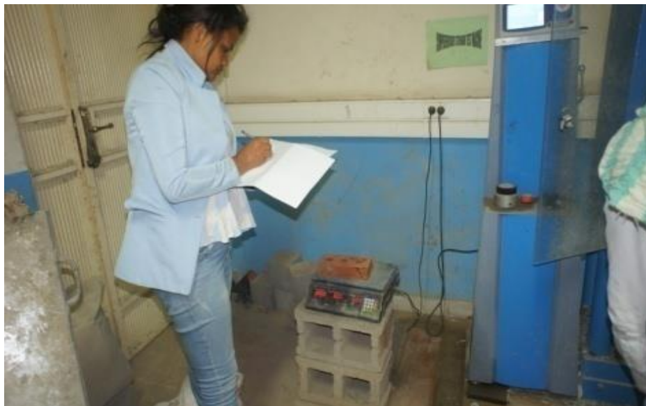
Figure B- 8: Compressive Strength Testing Process
