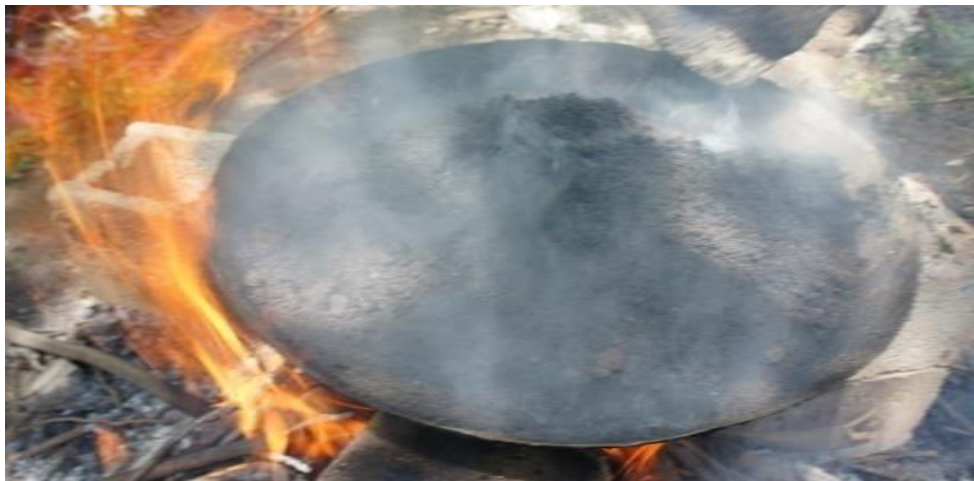
Figure B- 4: Mixing Process of Sand and Plastics
