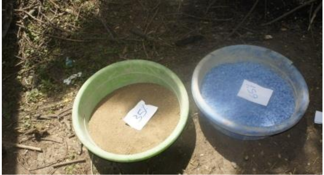
Figure B- 3: 35% and 65% Preparations of Plastic and Sand Respectively
