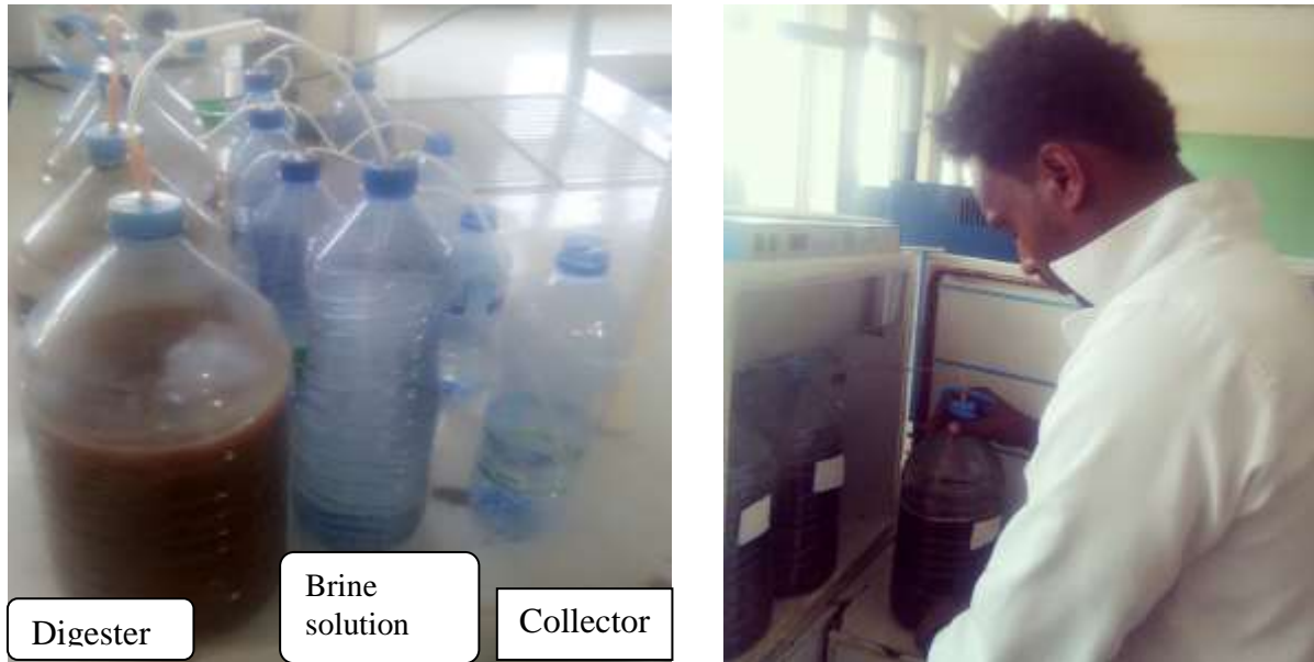
Figure 3: Experimental set-up of anaerobic digestion
