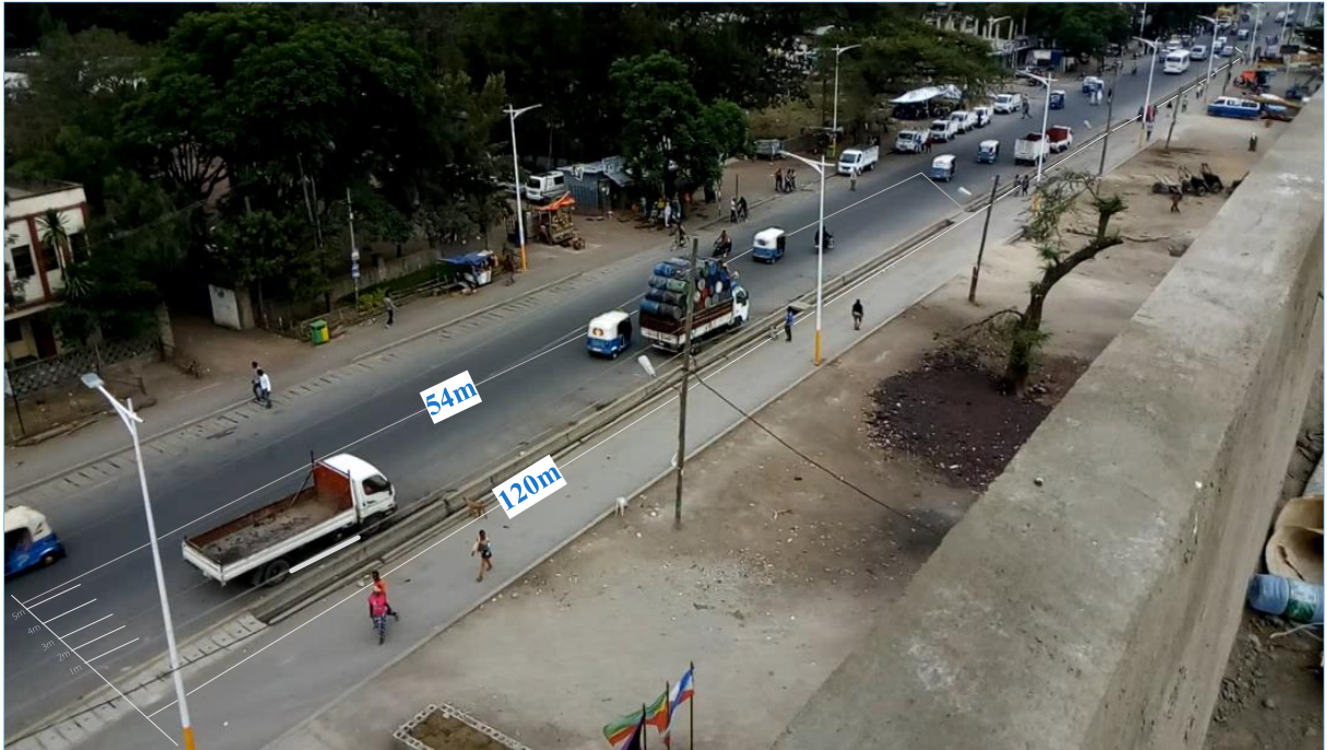
Figure 4-2: Spot Speed and On Street Parking Base lengths (54m and 120m respectively)
