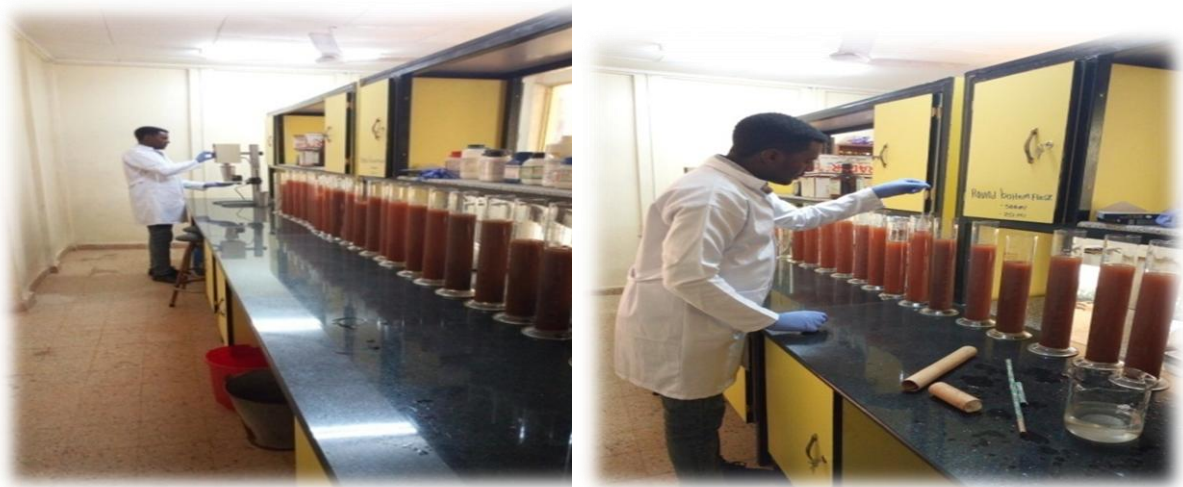
Figure 3.4: Soil textural class determination /Hydrometer reading in the laboratory
