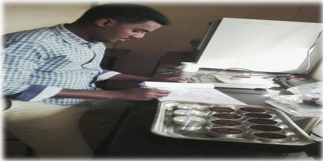
Figure 3.6: Soil moisture determination using oven dry method
