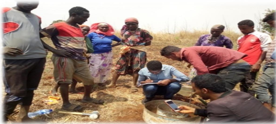
Figure 3.5: Infiltration test of the soil at field
