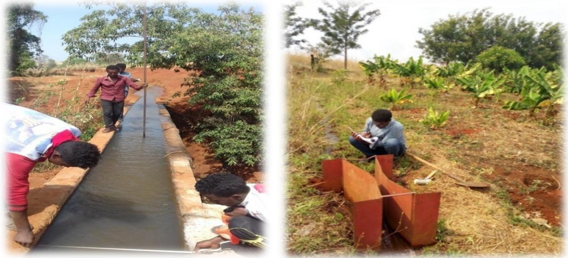
Figure 3.3: Determination of discharge, cross section and cross drainage structure
