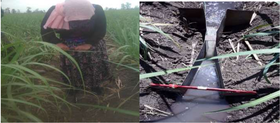
Appendix figure 3: Taking of soil sampling and Inflow measuremet
