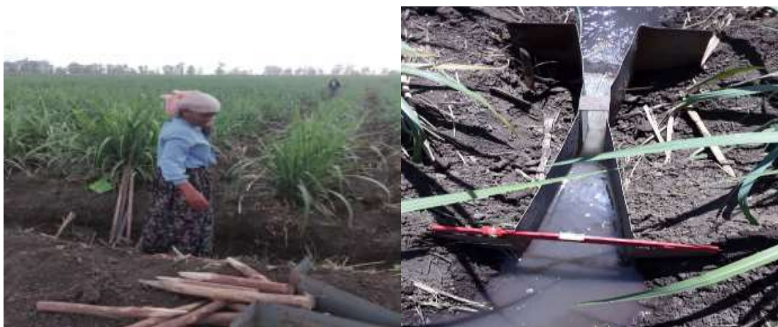
Figure 4: Inflow measurement with parshall flume
