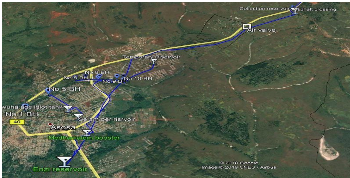
Figure 5. Arrangement of the wells and Conveyance system
