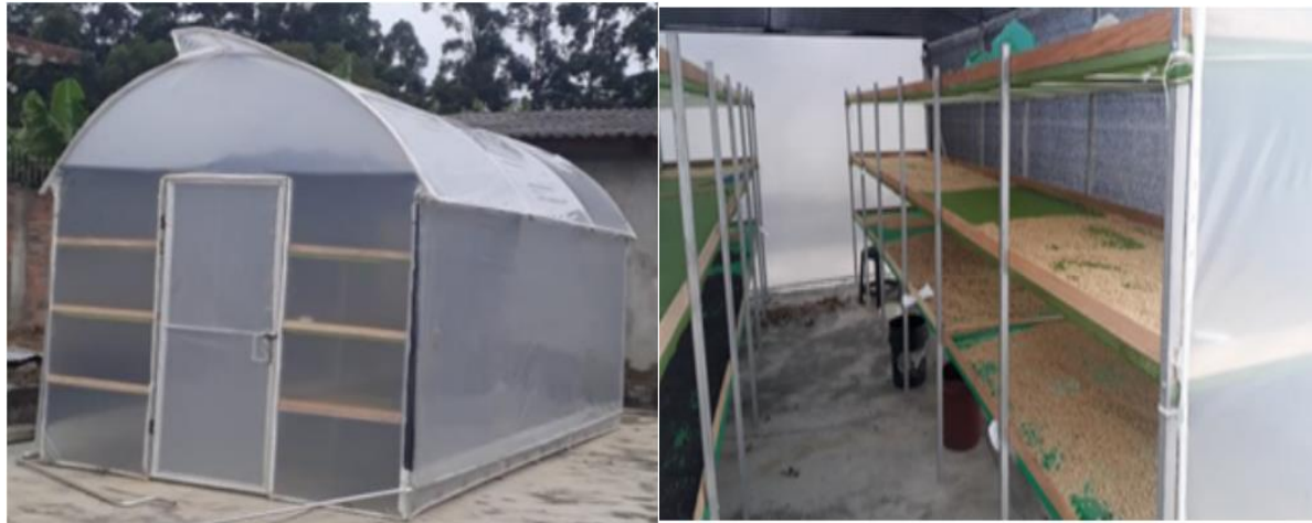
Figure 2.5 Greenhouse type solar dryer with drying beds by (Briceño-Martínez et al., 2020).
