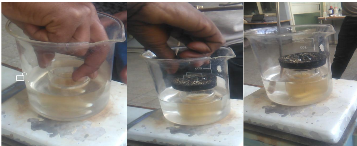
Figure 3. 4. Pictorial representation of the preparation of copper oxide thin films
