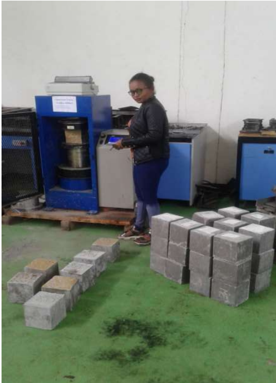
Figure B. 4 Compressive strength test cube specimens
