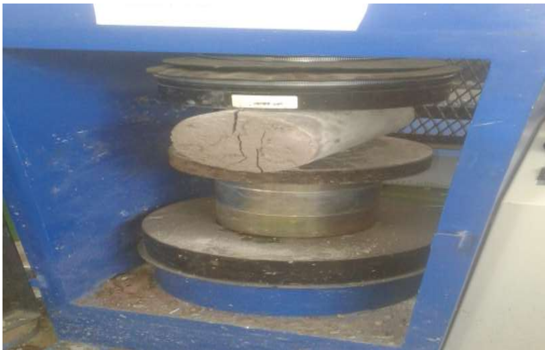
Figure B. 7 Tensile splitting test
