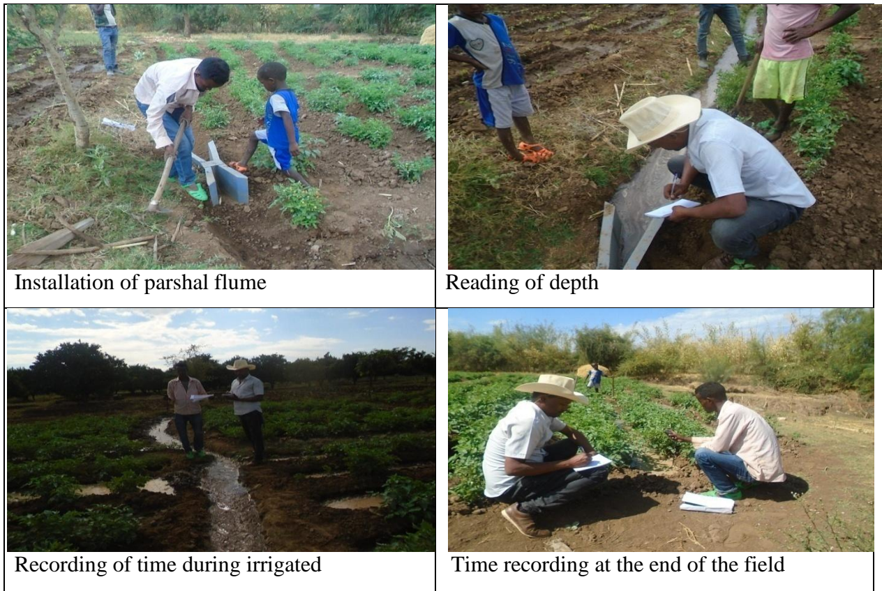
Figure 3.8: Measurement of Flow rate in field through Parshal flume
