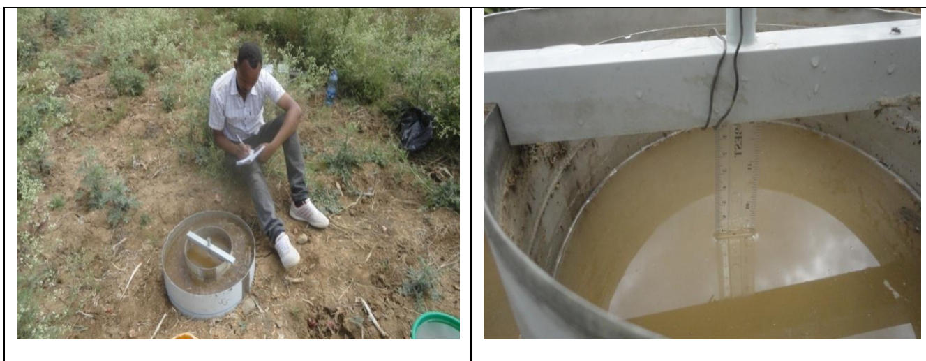
Figure 3.6: Measurement of infiltration rate
