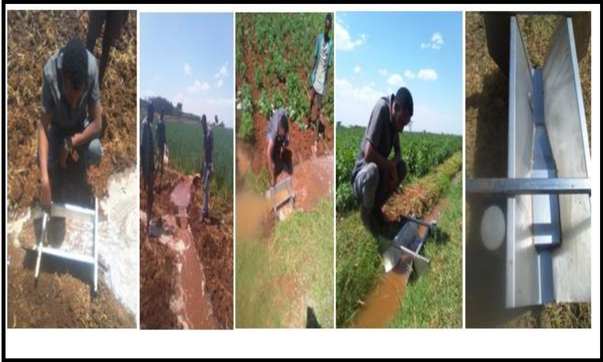
Appendix Figure 2: Field water application depth and discharge measurement with RBC flume.
