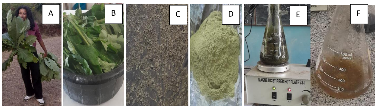
Figure 7: Block diagram of S. gigas extract synthesis ; sample collection (A), Washing (B), Drying (C), S. gigas powder (D), Heating (E), Filtration and Filtrate (F)
