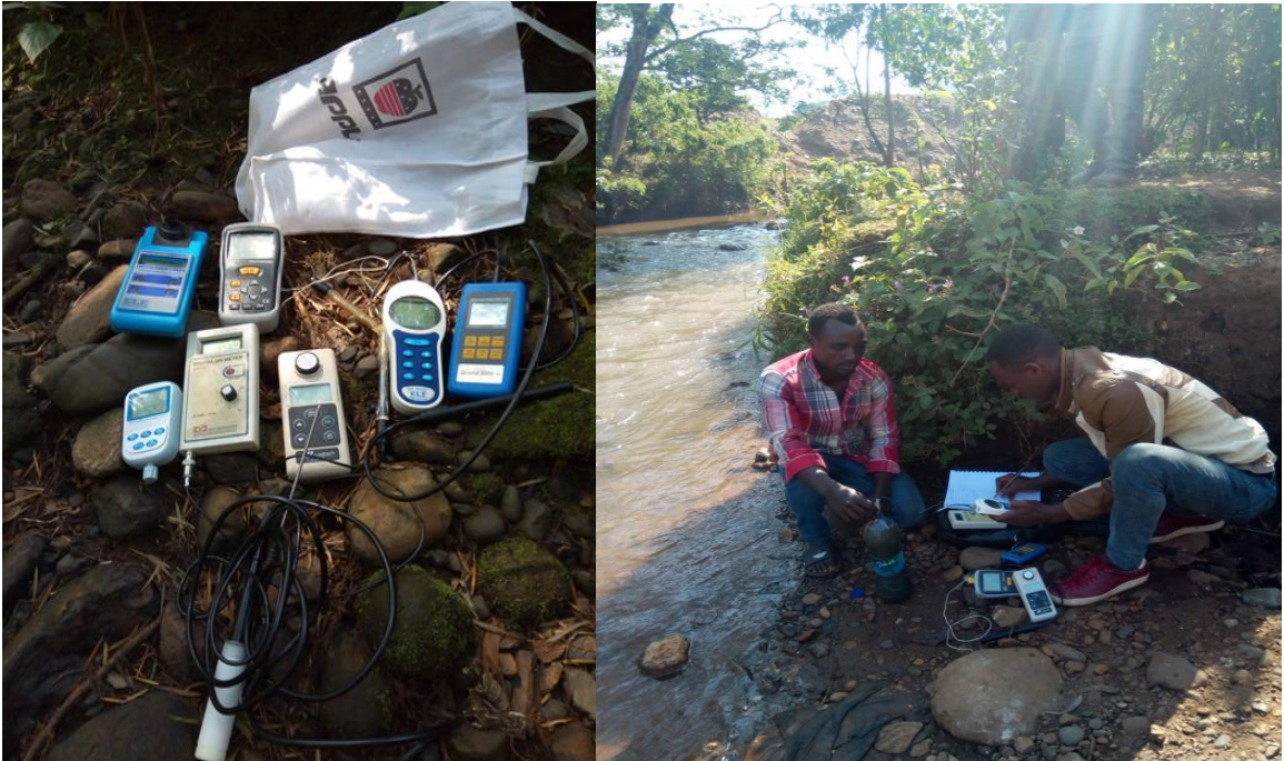
Figure a 1: Collected instruments and onsite measurement of the selected quality parameters
