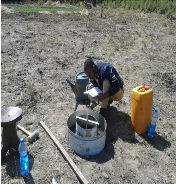
Figure 3.3: Soil infiltration measurement
