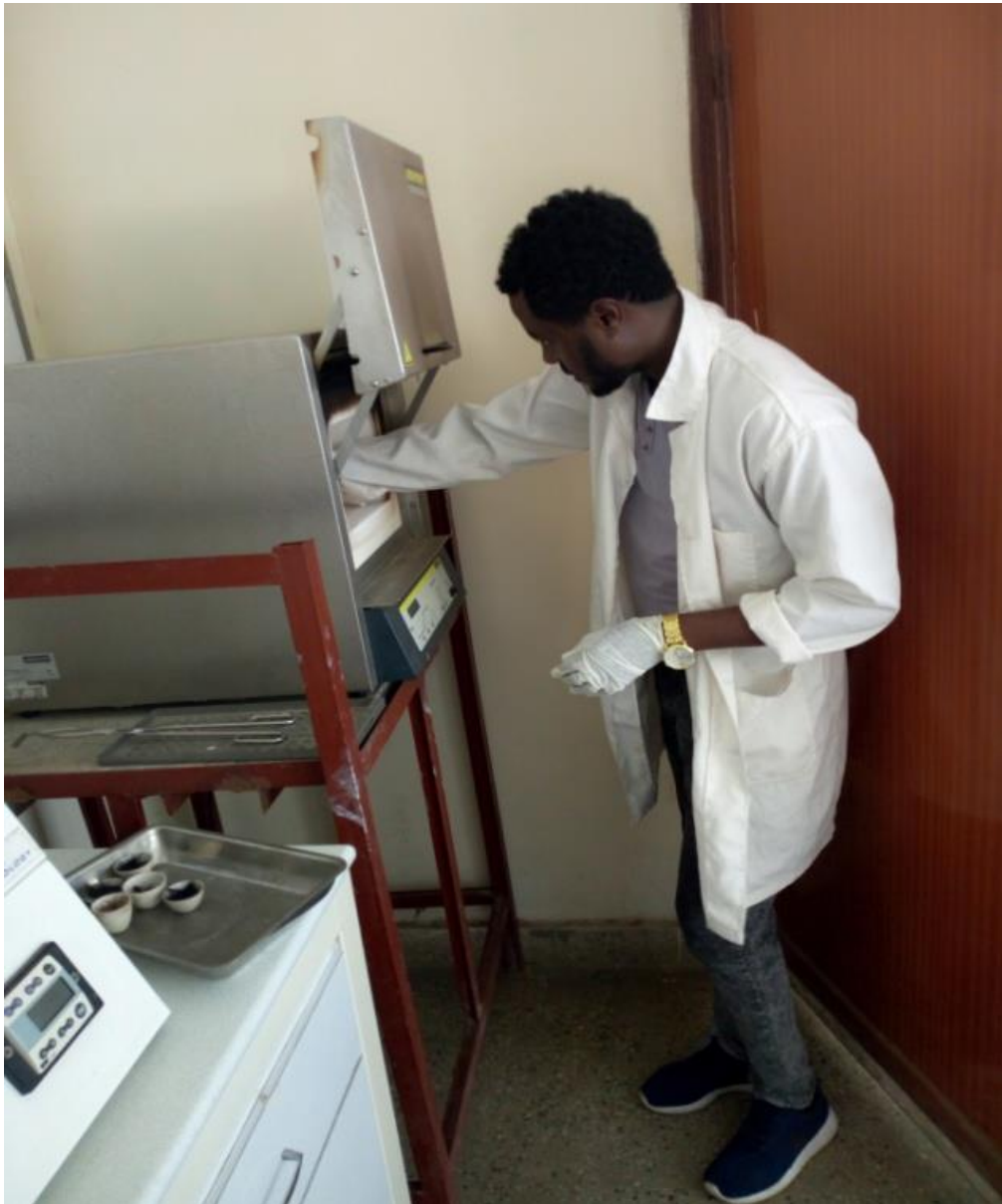
Figure 8 Analysis the ash content of the fibers
