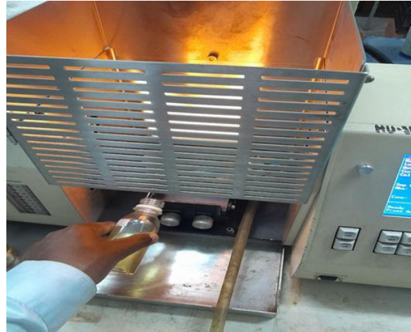
Figure4: Sample taken to the nebulizer (to atomize)
