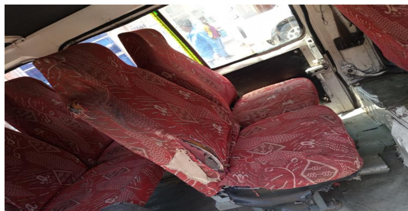
Figure:3.3.minibus taxi internal chair defect and appearance
