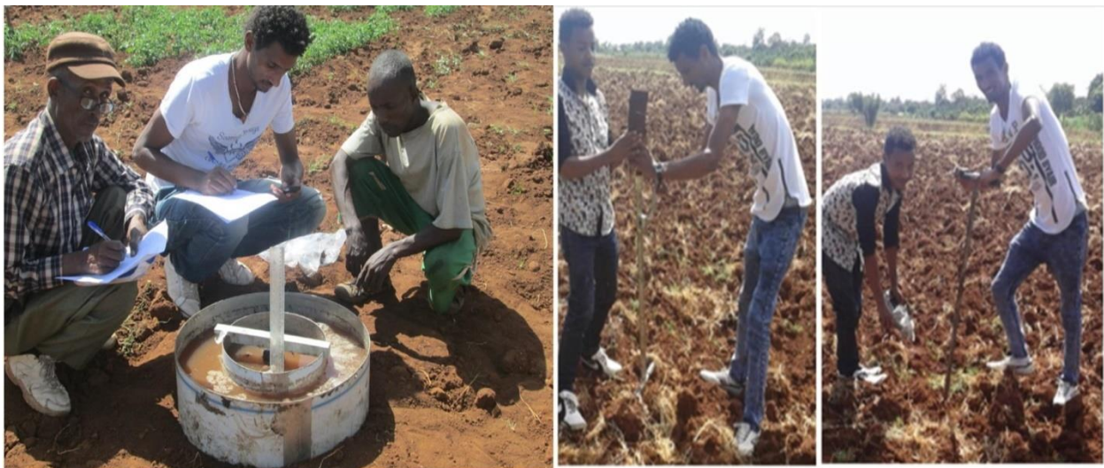
Figure 3: Measuring Soil Infiltration Rate and Soil Sampling
