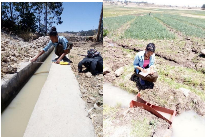
Figure 3. 3:Determination of cross section of the canal and field discharge using parshall flume
