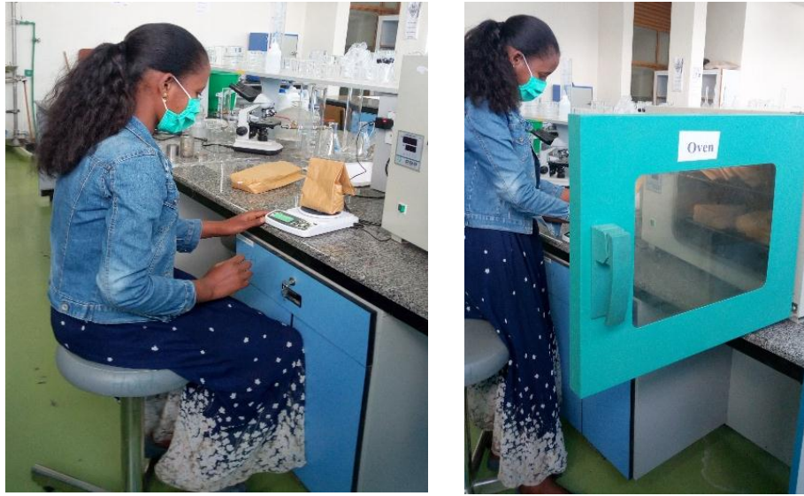
Figure 3. 5: Soil moisture determination using oven dry method.
