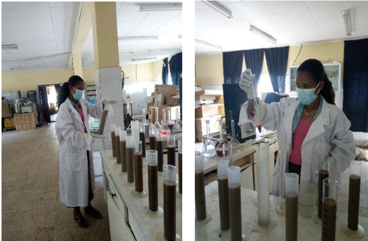
Figure 3. 4: Soil texture determination using Hydrometer
