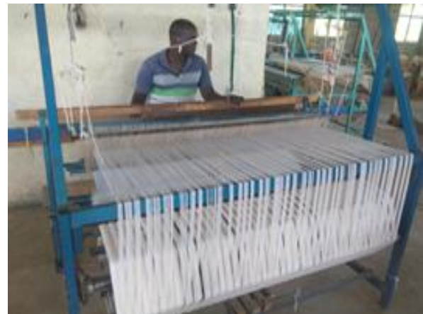
b. Modified loom- with maximum production rate 1.5m wide & 1.5m per hour = 2.25m 2 /hr
