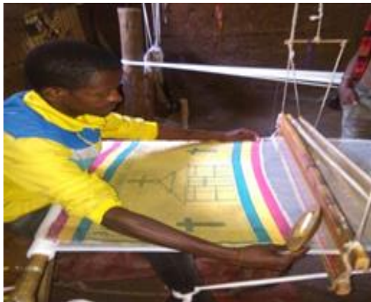
a. Traditional loom- with maximum production rate 1m wide & 1m per hour = 1m 2 /hr
