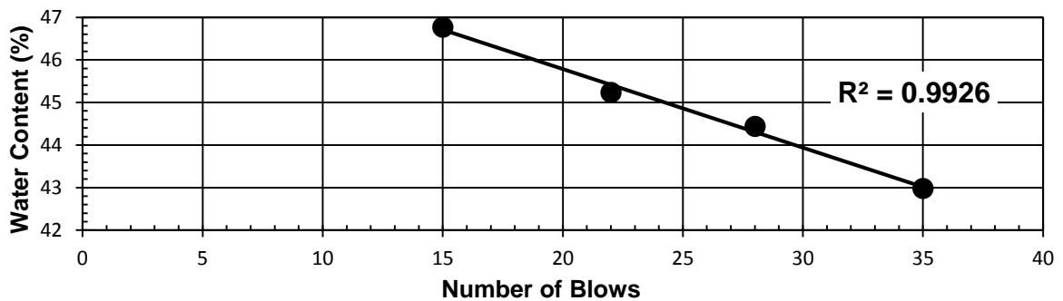
Figure A 2.1: Graph of water content versus number of blow for untreated soil sample.
