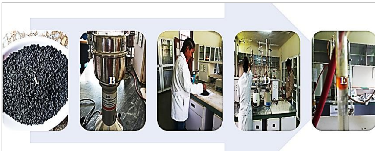
Figure 4.2. Essential and fixed oil extraction process: A) Black cumin seeds, B) Seed grinder, C and D) Ground the seed, put it in the flask containing water, and assemble the Clevenger apparatus, respectively, and E) The extracted essential oil in the flask.
