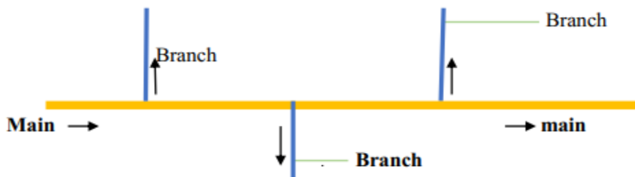
Figure 2. 3: Branched or Dead end system
