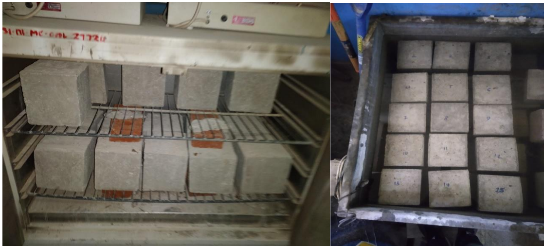
Figure 3.6: Cube specimens for water absorption test
