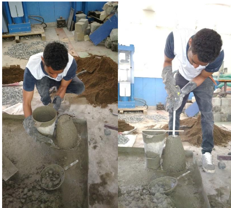
Figure 3.3: Slump apparatus and slump test
