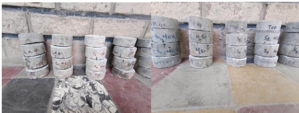
Figure 3.7: Sorptivity test specimens after cutting the parent cylinders.
