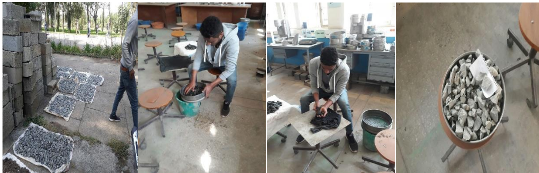
Figure C 2: Washed aggregate and specific gravity test on coarse aggregate
