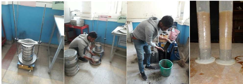
Figure C 1: Sieve analysis, specific gravity & silt content tests on sand
